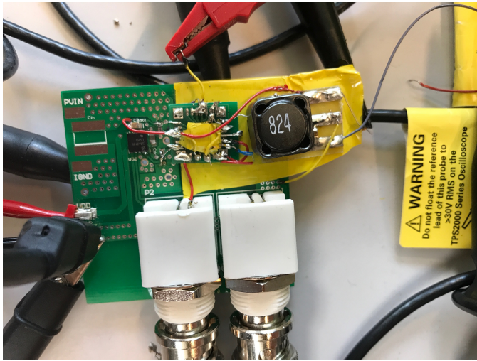
Fig. 8. Photograph of the implemented synchronous buck prototype with the test chip under yellow isolation tape, the gate drive signals fed through the white BNC connectors at the bottom and the output inductor on the right side.
