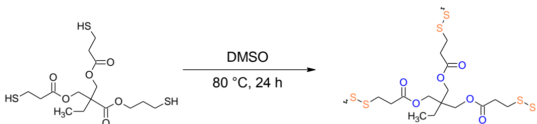
Figure 2.5 Polymerisation scheme of disulphide polymer, COP-65.
