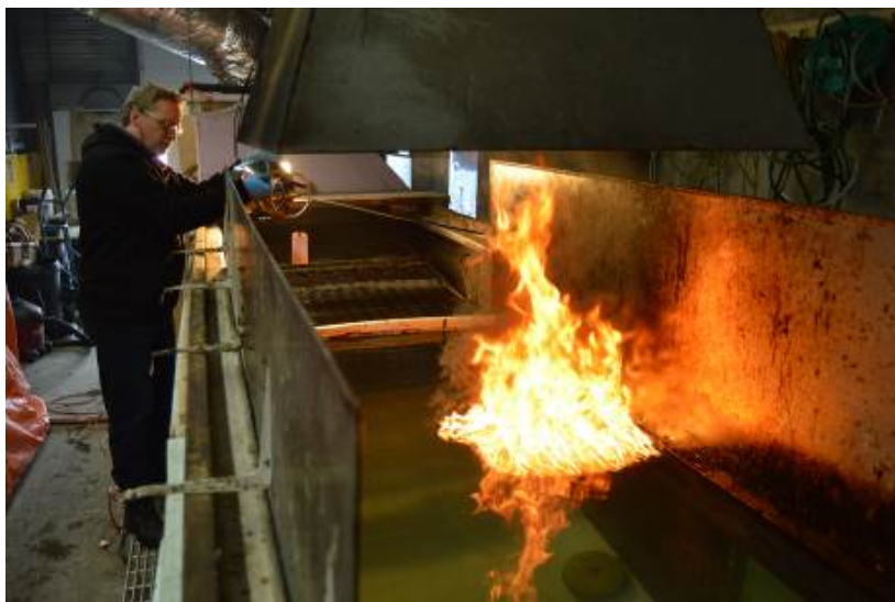
Figure 7 Herded slick burning under fume hood suspended over wind/wave tank
