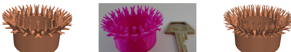
Figure 1: Designs generated using topology optimization are shown. An objective function related to heat conduction gives a hairy design with more or less branching (right or left). A preliminary extrusion based on fused deposition modeling is shown in the center. Currently, there are no plans for in vivo testing.
