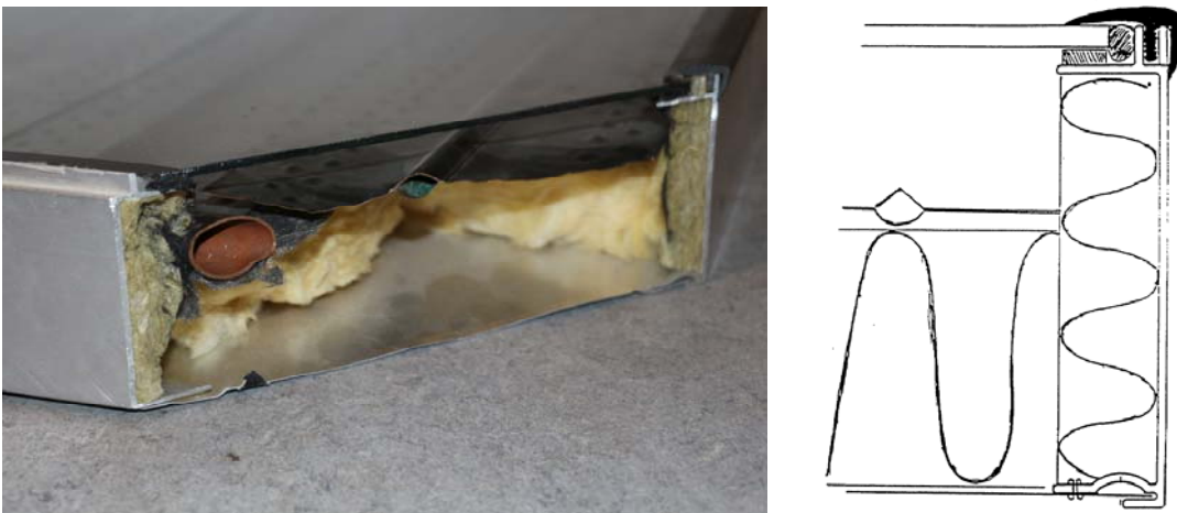
Figure 7. Picture and schematically drawing of the solar collector design.
