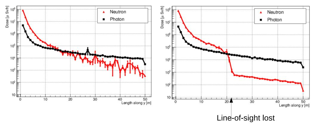
Dose-rates, measured 5cm in the steel converted from flux according to official Swedish radiation protection procedures
