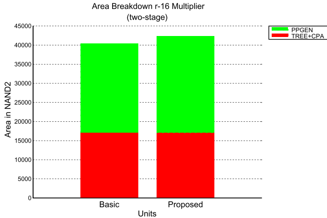
Fig. 9. Area breakdown for 2-stage pipelined multipliers.
