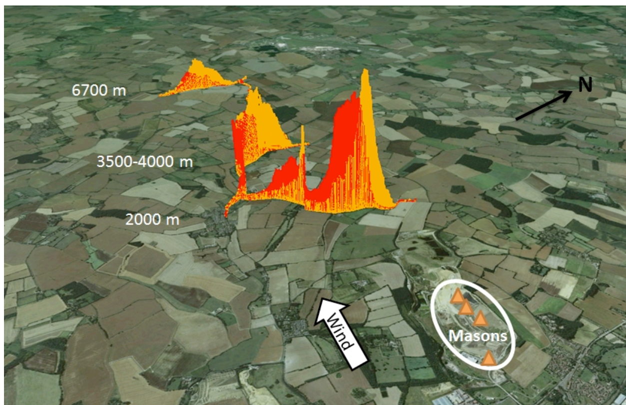
Figure 1. Relative atmospheric methane (red) and acetylene (yellow) concentrations above background measured at three different distances to the landfill on road W1, 2 and 3 on Aug. 7 th , 2014. Maximum methane concentrations above background were 2620, 1290, and 590 ppb at the three measuring distances 2000m, 3500-4000m and 6700m, respectively. Maximum acetylene concentrations above background were 15.2, 9.0, and 4.6 ppb at the three measuring distances 2000m, 3500-4000m and 6700m, respectively. Yellow triangles mark the approximate placement of the tracer gas bottles). Map data: Google, Infoterra Ltd & Bluesky.
