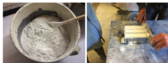
Fig. 3. Mixing and casting of prisms and cylinders
