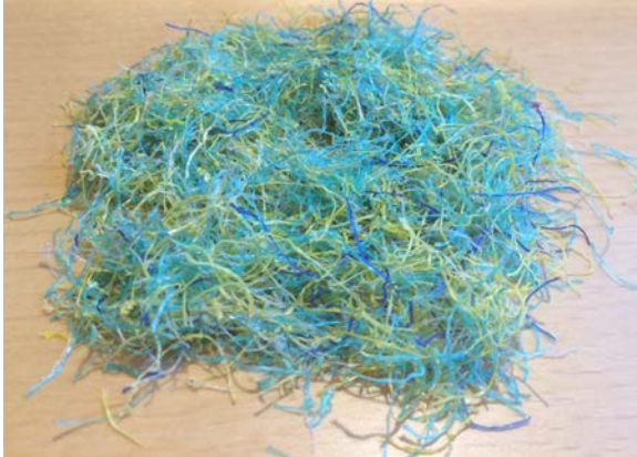
Fig. 1. Monofilament fibres of polyethylene by Plastix A/S produced by mechanical cutting operation
