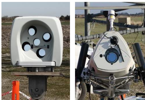
Figure 1. The two nacelle lidar systems used in this study and the Nørrekær Enge campaign: five-beam Demonstrator (left) and ZephIR Dual Mode (right).
