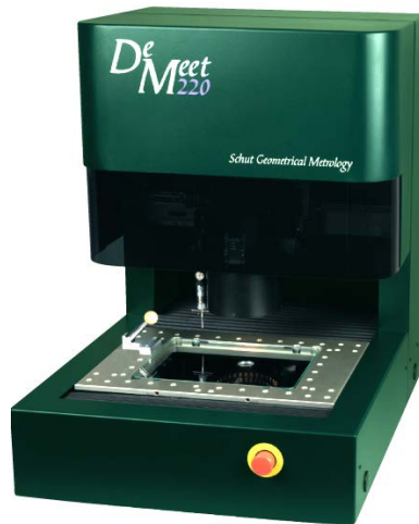
Figure 5.3-2. Optical coordinate measuring machine (DeMeet 220 – OCMM) used in the investigation.
