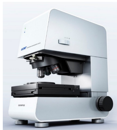
Figure 4.4-3. Optical instrument used in the investigation: Olympus Lext OLS 4100 (laser scanning confocal microscope – CM).
