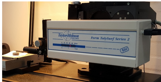
Figure 4.2-3. Reference instrument: Taylor Hobson Form Talysurf series 2 Inductive 50.
