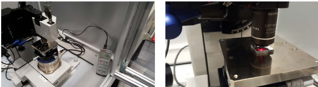
Figure 8.5-1. Mitaka MLP-3SP in its housing chamber (left). Detail of stage hosting the optical flat used in the investigation (right).
