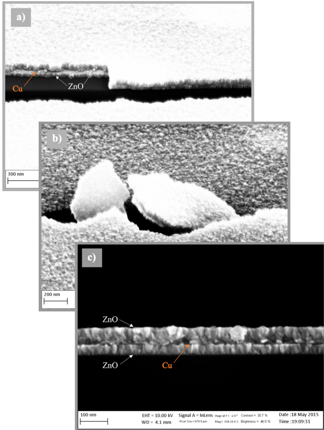
Figure 7.4: SEM images of a ZnO/Cu/ZnO sandwich structure.
