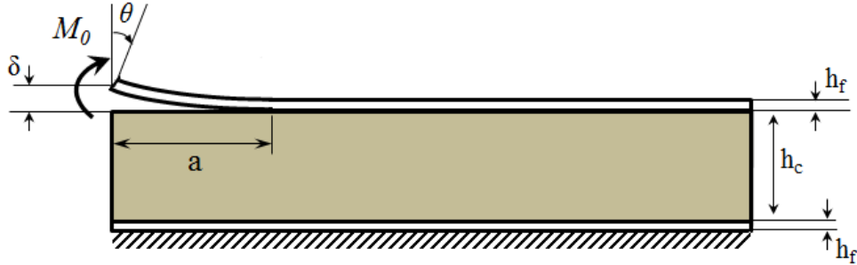
Figure 3. Moment-loaded SCB specimen.
