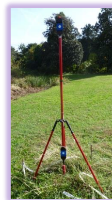
Figure 9: Leica target pole used for traversing with the C10
