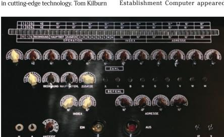
FIGURE 6 – The control panel of the Mailüfterl, completed by Heinz Zemanek in 1958. The design, started four years earlier, was an early transistorized computer. (Photo courtesy of Wikimedia Commons.)
