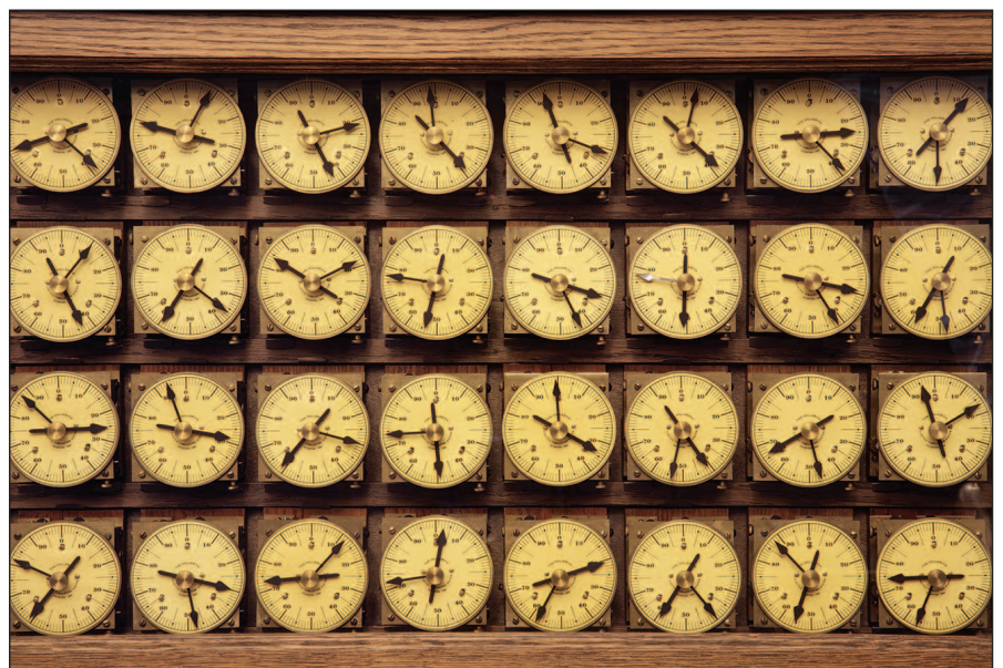
FIGURE 1 – The counter dials of the Hollerith tabulator first used for U.S. census data processing, 1890. (Photo courtesy of Wikimedia Commons.)
