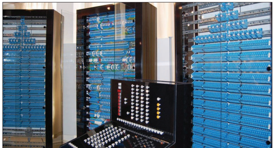
FIGURE 5 – A replica of Zuse's Z3. The machine was operative in 1941. (Photo courtesy of Wikimedia Commons.)
