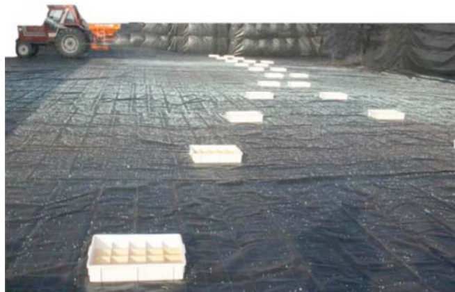
Figure 3 Physical tests carried out for determination of actual distribution at boundary conditions
