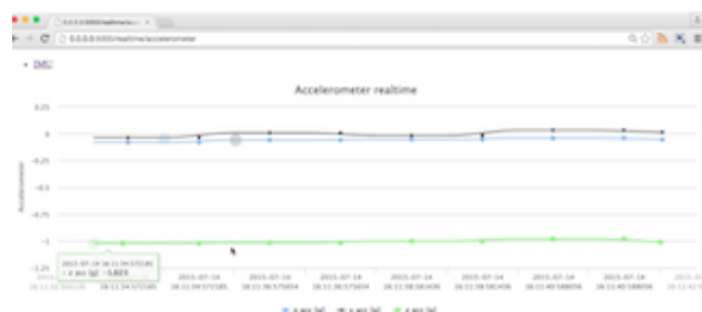
Figure 6. An example of real time measures from the inertial navigation sensor.
