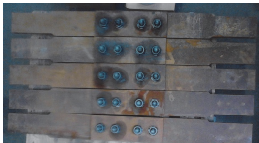
Figure 6: Blasted and rusted specimens.
