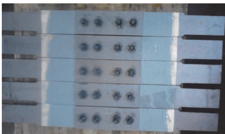
Figure 11: Blasted and half-coated specimens.
