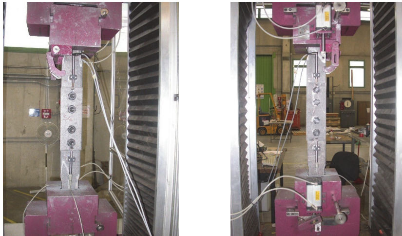
Figure 3: Test of the blasted specimen.
