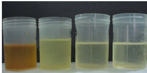
Figure 01. Extracts obtained from sequential treatments of soil samples for organic matter removal with sodium hypochlorite (NaClO) pH 9.5 (adapted from Anderson [7]). Seropédica, RJ, 2009.
