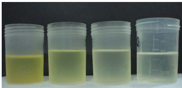
Figure 01. Extracts obtained from sequential treatments of soil samples for organic matter removal with sodium hypochlorite (NaClO) pH 9.5 (adapted from Anderson [7]). Seropédica, RJ, 2009.
