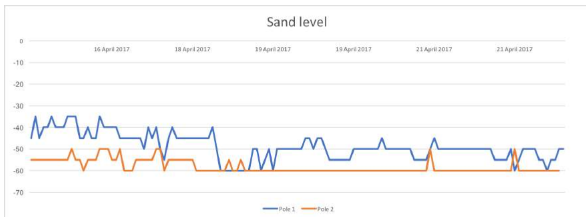
Figure 8. Sand level variation trends measured by the two poles.
