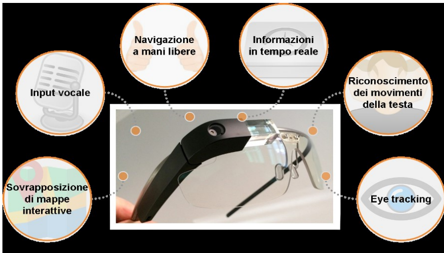
Figura 8. Functional features of Google Glass.
