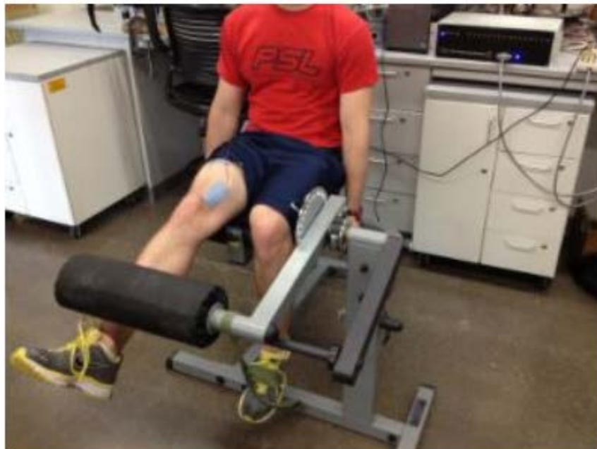
Figure 13 A subject sitting in a leg extension machine with surface electrodes on the quadriceps muscles.
