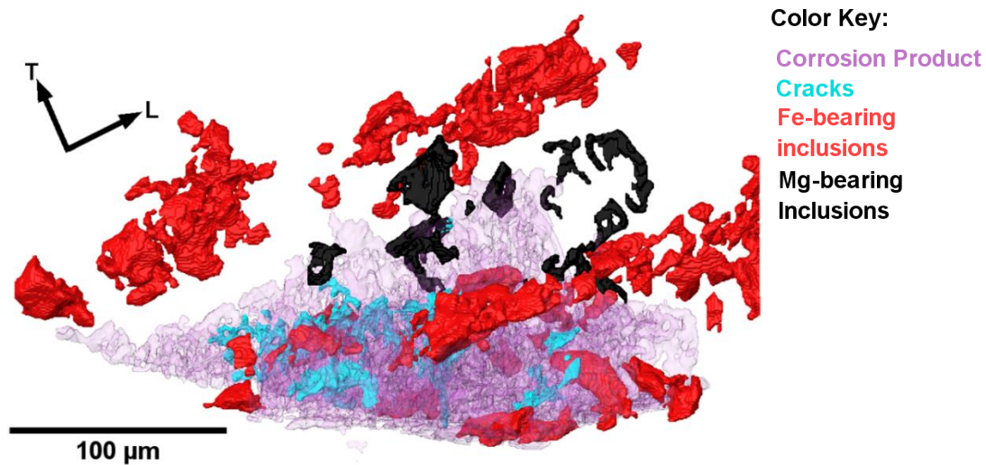
Figure 5: L-T view of the crack-initiating crevice corrosion pit. The pit has a sharp geometry which serves as a stress concentration for fatigue crack initiation and growth.
