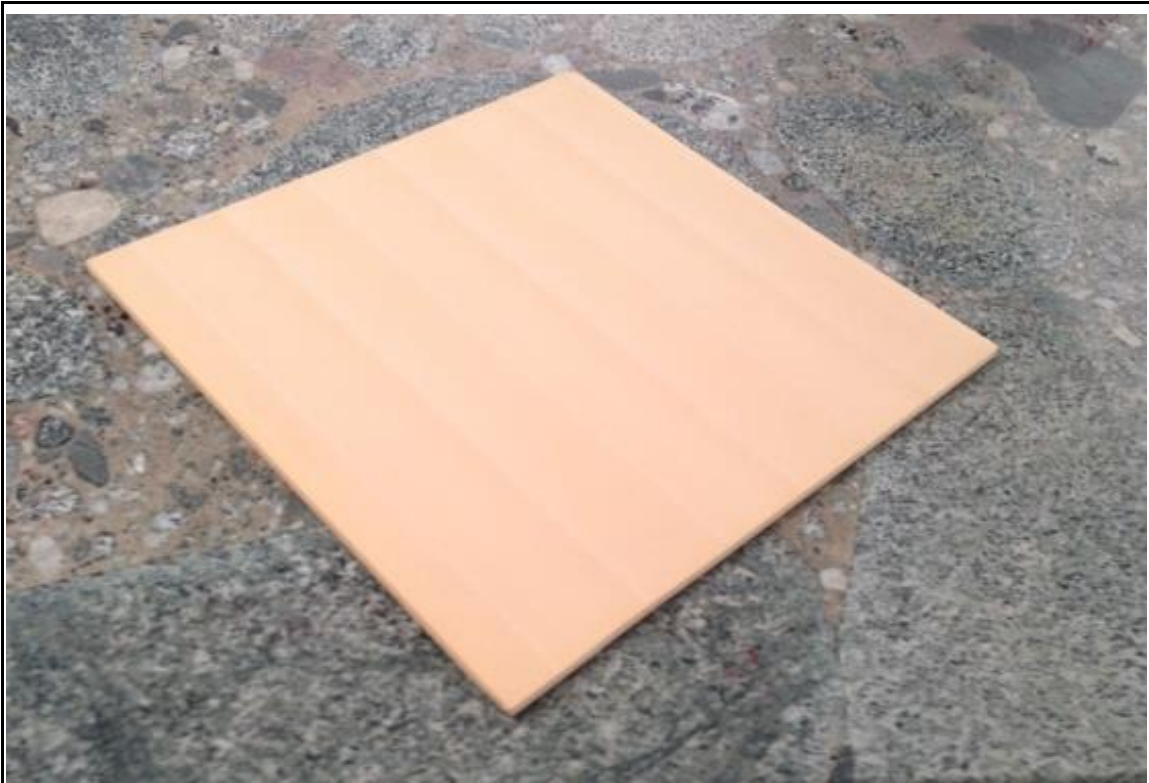
Figure 9-7. Diab HCP70 \epsilon_r = 1.39 . Foam Top Matching Layer.
