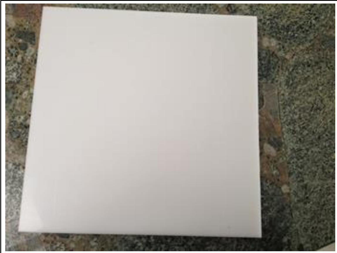
Figure 9-8. HDPE \epsilon_r=2.33 . Second Matching Layer.
