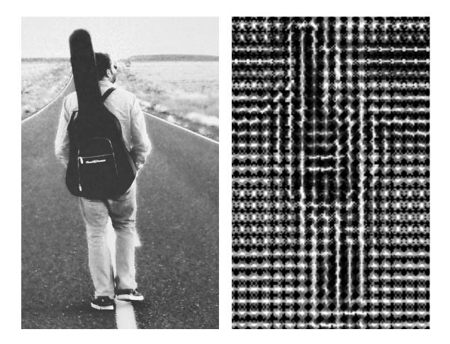
Figure 1.2: Histogram of Oriented Gradients
