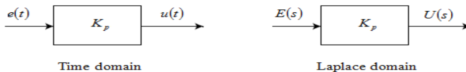
Figure 5.5: Representation of the proportional controller in the time and frequency domains
