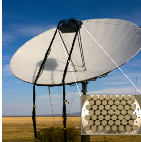
Figure 4: MIDAS detector installed in the Pampa at the Pierre Auger Observatory.
