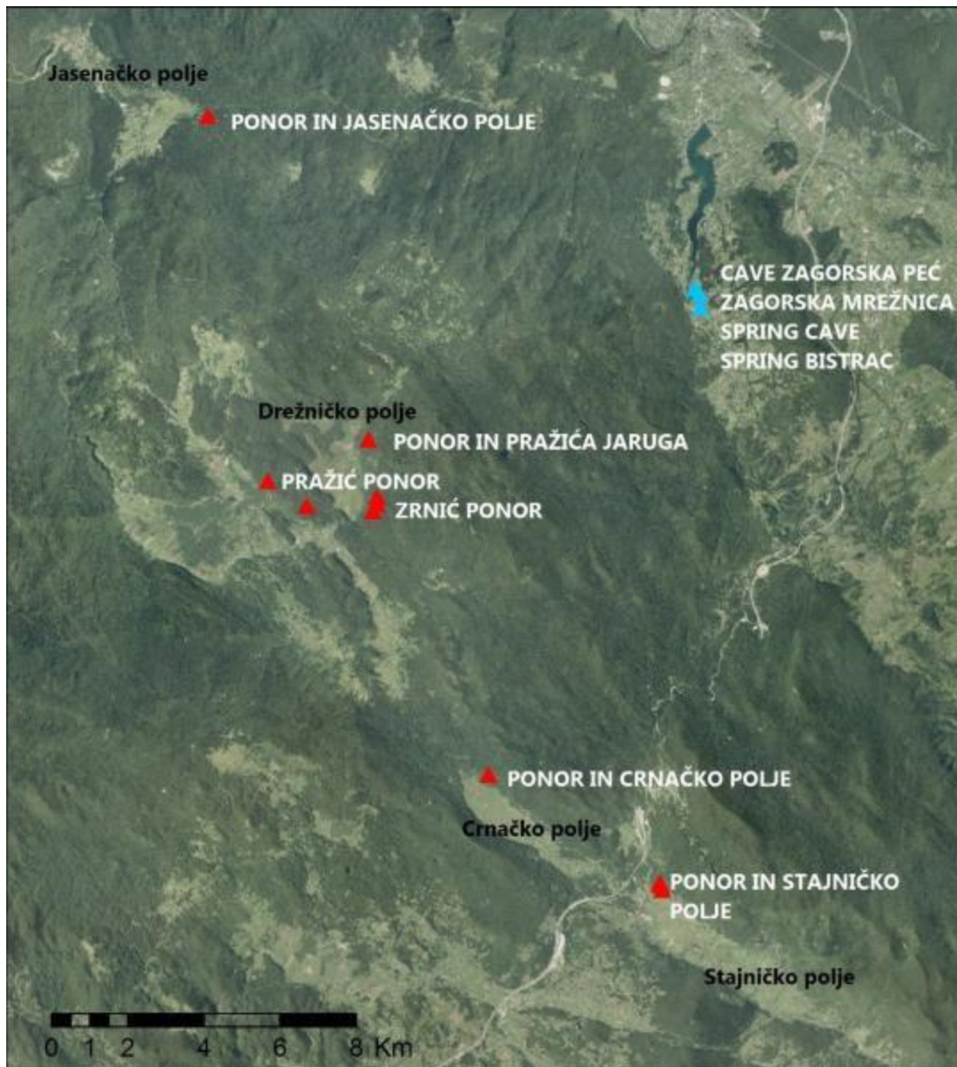
Figure 16: Ponders in which the tracing method using fluorescein was done and springs where the connection was proven.
