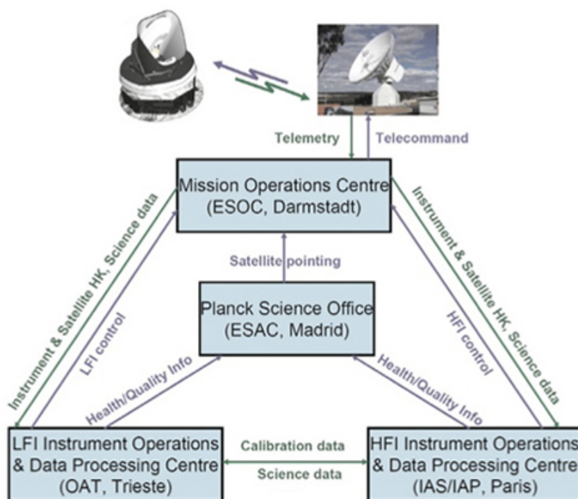
Figure 3.7: A sketch of the centres involved in the Planck ground segment and the main data exchanges between them
