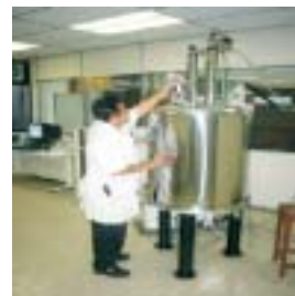
Encik Jasmi, Lab. Assistant operating the Nuclear Magnetic Resonance (270 MHz FT-NMR) Spectrometer
