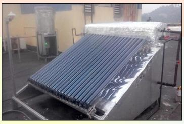
Experimental setup of SWH system and the structure of thermal battery
