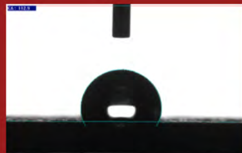
Figure 2: Maximum contact angle more than 130° achieved by the developed coatings
