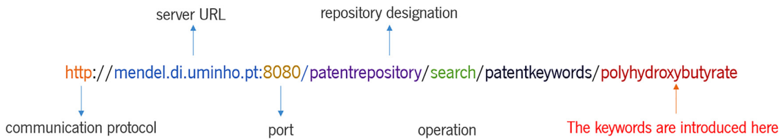
Fig. 4. Example of the used URI to access the local repository with patent from USPTO since 2005, searching for patents using specific keywords.
