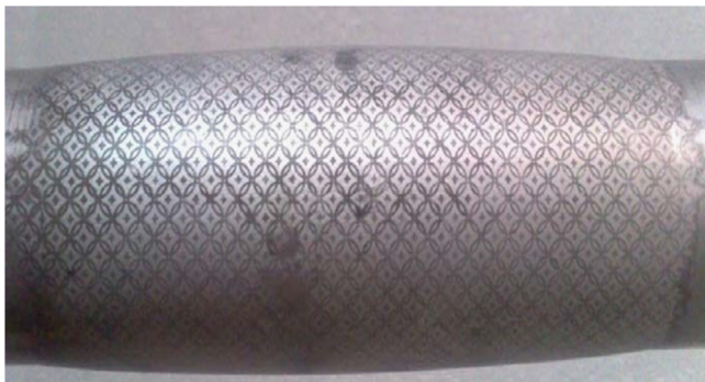
Fig. 4. Grid patterns etched onto tube's surface for experimental measurement of surface strains.
