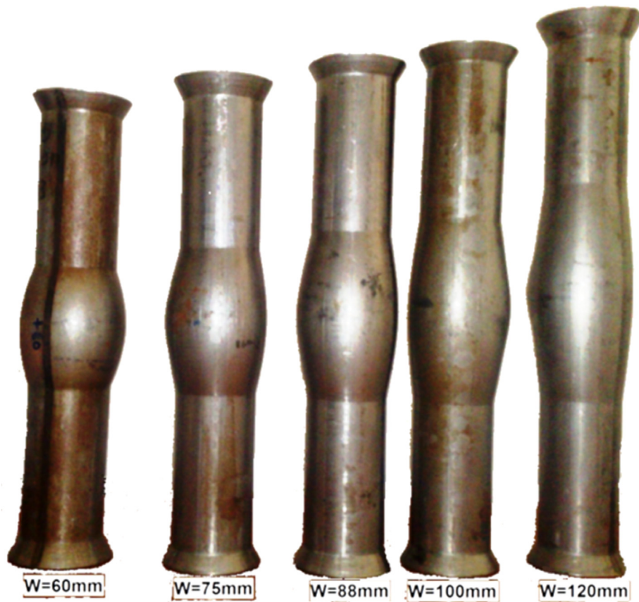
Fig. 2. Free hydroformed parts for different bulged widths.
