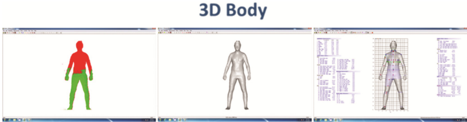
Fig. 3. Image software stages: data cloud image, reconstructed surface image, image with measurements – 3D body scanner software
