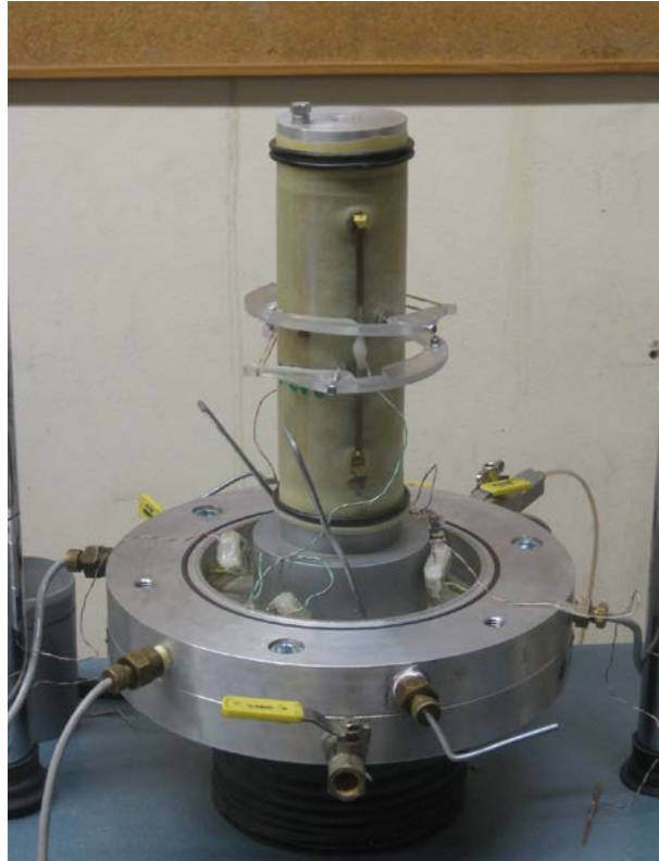
Figure 5: Triaxial test setup showing Linear Displacement Transformers (LDT) instrumentation
