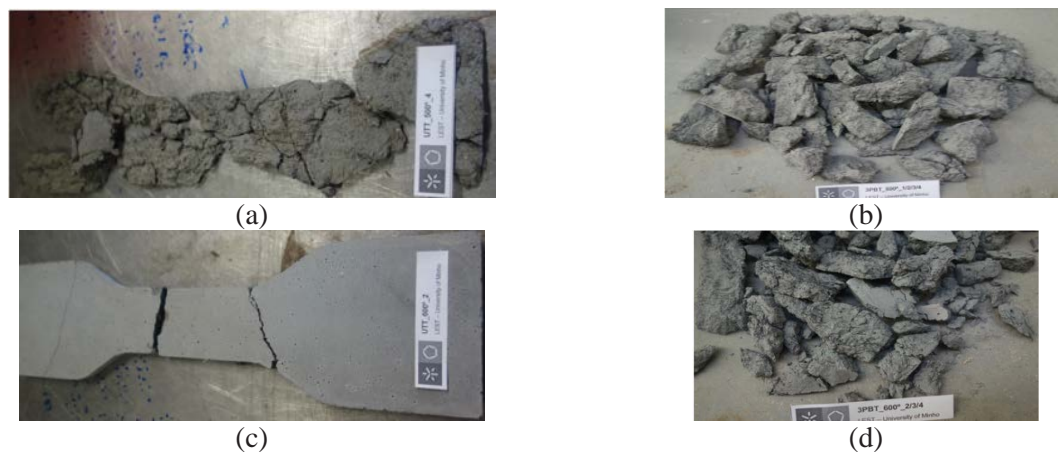
Figure 2. Failure due to high temperature: (a) and (b) spalling at 500 °C of direct tension and flexure specimens, respectively; (c) cracking of direct tension specimen at 600 °C, and (d) spalling of flexure specimens at 600 °C.
