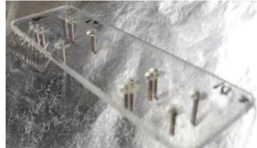
Fig.3 – Device fabricated by a micromilling machine and sealed with an adhesive film.
