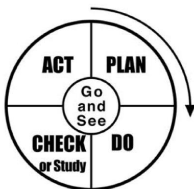
Figure 2: Toyota added the words "Go and See" to the PDCA cycle (adapted from Rother, 2009)
