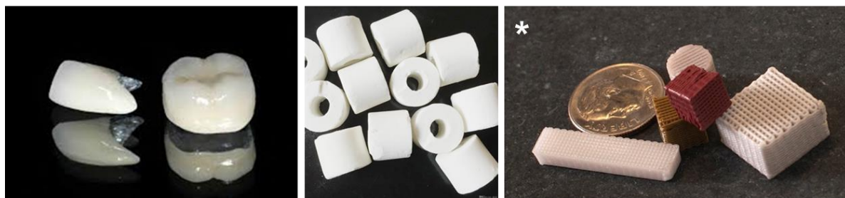
FIGURE 2. Bioactive glass and glass-ceramics for biomedical applications and porous robocast bioglass produced at Missouri University of Science and Technology for bone repair and regeneration (*) (54, 55).
