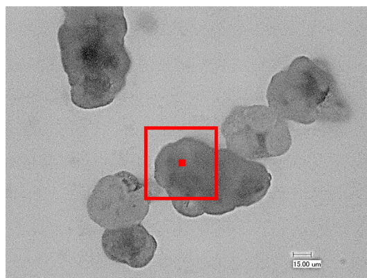
Fig. 14. Light microscopy image of PAMC before their insertion into the microfocus WAXS beamline. The small solid square depicts the size of the WAXS microfocus related to the sample area scanned (the big square) and the size of the loaded PAMC.
