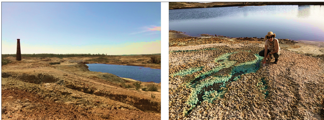
Figure 2 – Image of PAT 7 surrounded by waste-dumps and piles and the presence of soluble salts at the banks of dam. Green color is due to melanterite ( \text{FeSO}_4 \cdot 7\text{H}_2\text{O} ).
