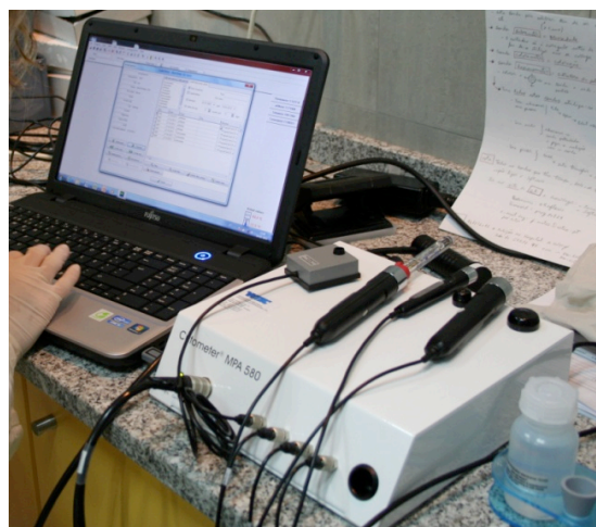
Figure 5: Cutometer MPA 580 used for evaluating the physical and chemical properties of the skin.
