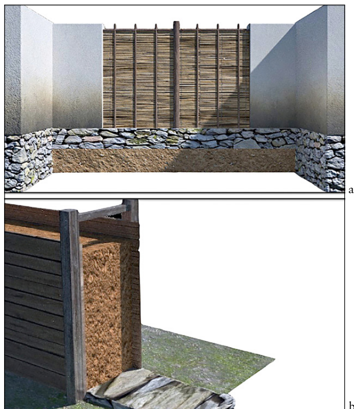
Fig. 1 – Construction techniques: a) Wattle and daub; b) Pisé.
