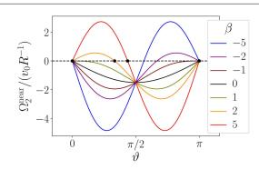
**Figure 4.** Wall-induced angular velocity of a squirmer from lubrication theory,  $\Omega_2$  of equation (12), versus  $\vartheta$  for different  $\beta$ . Stable fixed points ( $\Omega_2 = 0$  and negative slope) are indicated by black dots.
