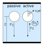
**Figure 2.** A passive particle sediments with a velocity  $v_1$  including the height-dependent friction coefficient. An active particle, in addition, moves with the swimming velocity  $v_0 \cos \vartheta$  along the vertical. Its self-generated flow field interacts with the wall and induces a deterministic linear  $(v_2)$  and angular  $(\Omega_2)$  velocity.
