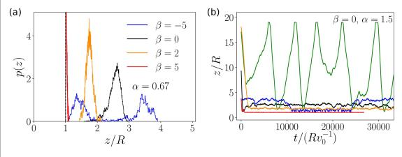
**Figure 1.** (a) Distribution p(z) of heights z during motion of a squirmer for  $\alpha = v_0/v_g = 0.67$  for different squirmer types  $\beta$  illustrating stable floating ( $\beta = 0$ , 2), wall pinning ( $\beta = 5$ ), and the bimodal state of recurrent floating and sliding ( $\beta = -5$ ). (b) Corresponding trajectories z(t). The green line illustrates a cruising state for  $\alpha = 1.5$  and  $\beta = 0$ .
