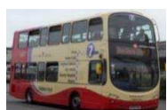
City Diesel-Hybrid Bus Engine: 161 kW + 120 kW (e.) EU V (DOC+DPF+SCR) City Line Profile
