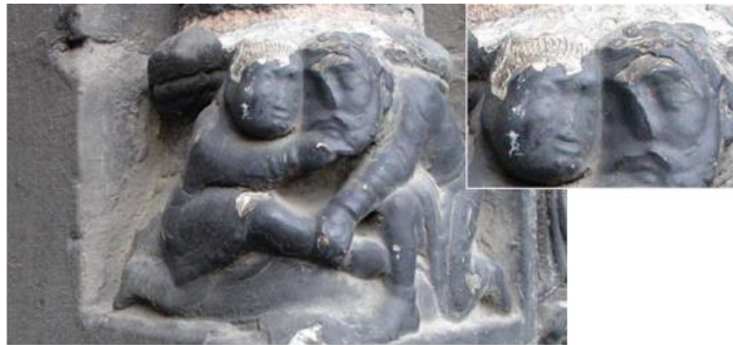
Figure. 1.1 - Black crust tracing the surface of a limestone sculpture, Saint-Denis -France [8].
