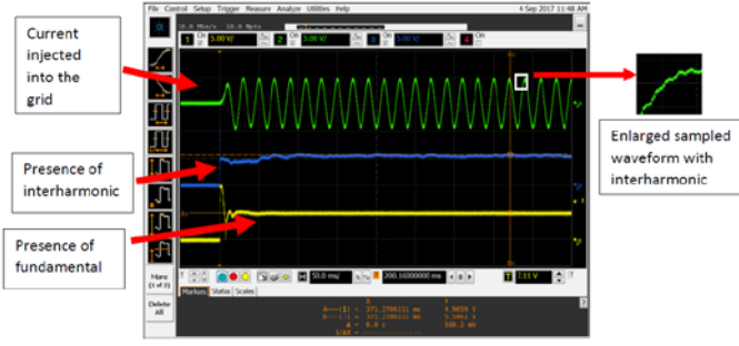
Fig.10 Current injected into the grid and the signals of the fundamental and interharmonic components (5V/div. for the three traces; 50ms/div.)
