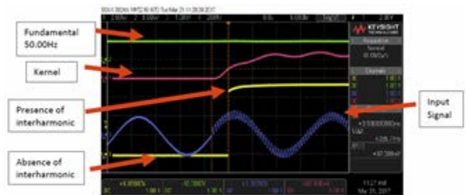
Fig. 5 Practical input signal with fundamental frequency of 50Hz superimposed with an interharmonic of 1.94kHz, and the analog versions of the computed fundamental and interharmonic frequency (5ms/Div.)
