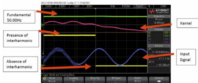
Fig. 6 Practical input signal with fundamental frequency of 50Hz superimposed with an interharmonic of 1.94kHz, and the analog versions of the computed fundamental and interharmonic frequency (5ms/Div.)
