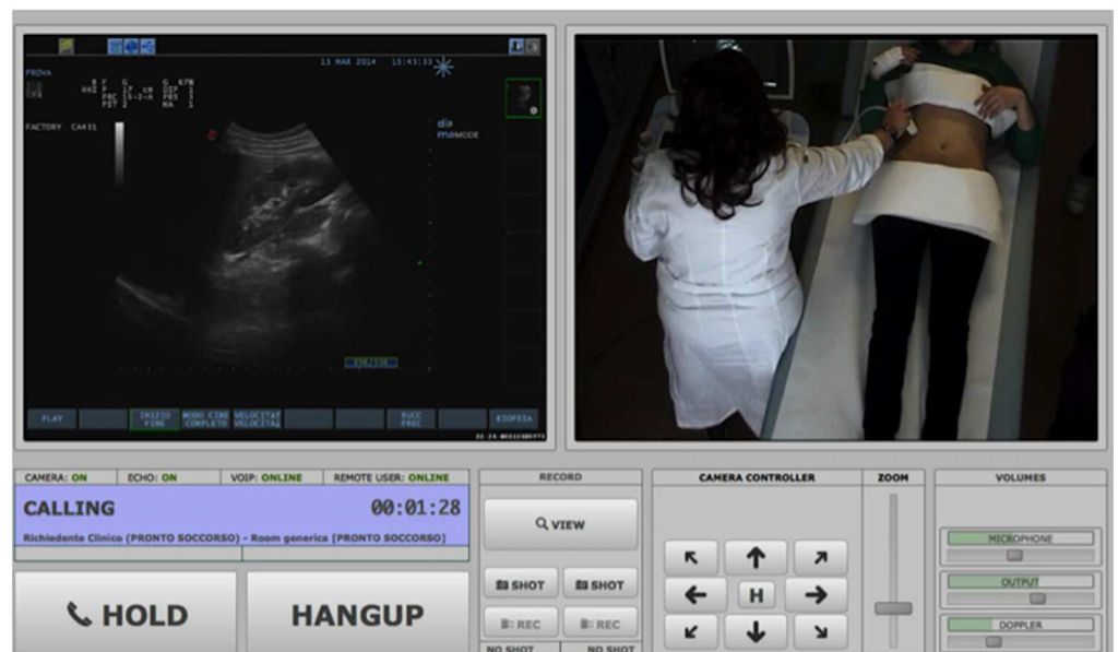
Fig 3. Detail of the images transmitted via tele-ultrasound, as appear on the radiologist's screen, also showing the buttons for remote control of the webcam, zooming functions and volume.
